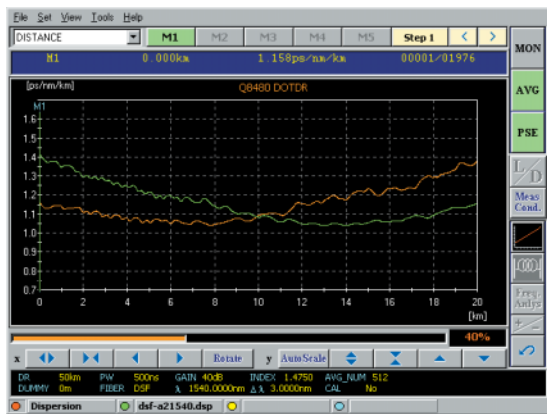
Figure 1: Dispersion Measurement Accuracy (Both Directions)
