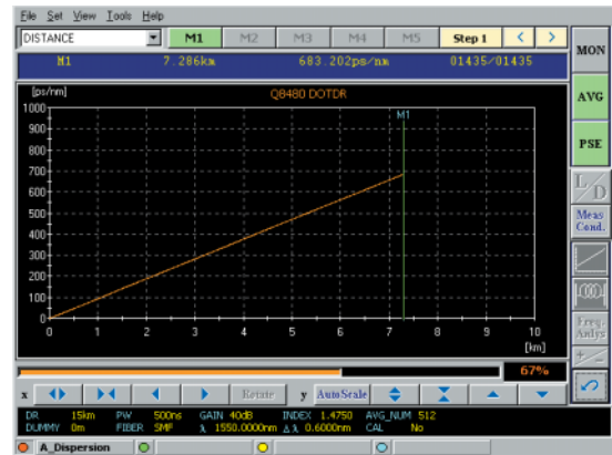
Figure 3: Measurement example of Dispersion-compensated fiber (Accumulative chromatic dispersion Display Function)
