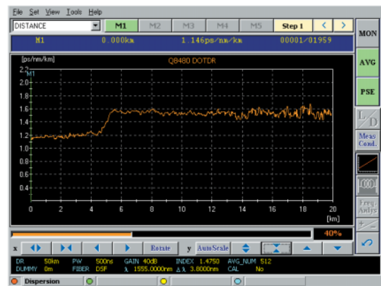
Figure 4: Measurement example of Connected Fibers with Different Dispersion Values
